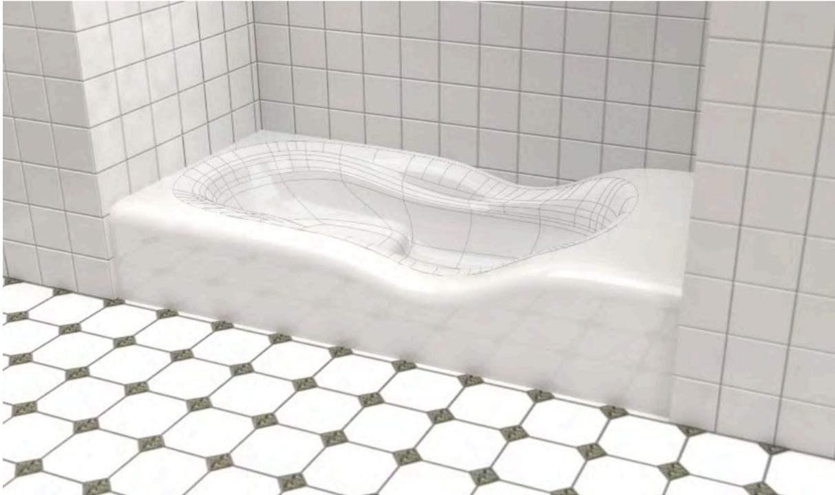
In this exercise, we will begin by creating a set of curves to define the contours of the bathtub. After lofting the curves to create a surface, we will then use a sequence of T-splines commands to add isolated detail, extrude a rounded bottom, add localized steps, apply symmetry, and match the T-spline surface with a trimmed NURBS.
